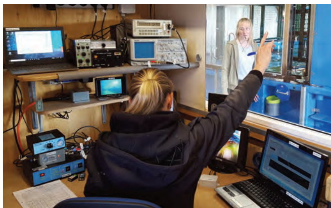
Research assistants and temporary hearing threshold test equipment at SEAMARCO. The equipment operator produces the fatiguing sound and watches for the California sea lion's reaction on a monitor. The trainer waits for a hand signal indicating whether the animal detected the sound and can be rewarded with a fish.
